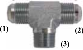
(1) JIC male, (2) JIC male, (3) NPTF male Parker STX-S SAE# 070425 Parker 213T Aeroquip 2030 (Reversed) Weatherhead C5605
