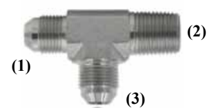
(1) JIC male, (2) NPTF male, (3) JIC male Parker RTX-S SAE# 070424 Parker 013T Aeroquip 2028 (Reversed) Weatherhead C5755
